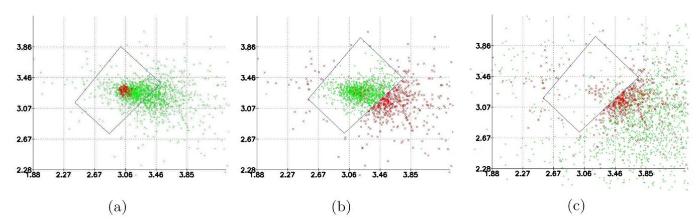
SIR algorithm: example. Figure (a) shows in red samples of the probability distribution  $p(\mathbf{x}(k-1))$  and in green the N particles  $\mathbf{x}^{j}(k)$ , j = 1, ..., N. Figure (b) shows time k+1. The target was not detected In green we have again the N particles  $\mathbf{x}^{j}(k)$  while in red the resampled N particles  $\tilde{\mathbf{x}}^{j}(k)$ . Figure (c) shows in red  $\tilde{\mathbf{x}}^{j}(k)$  and in green  $\mathbf{x}^{j}(k+1)$
